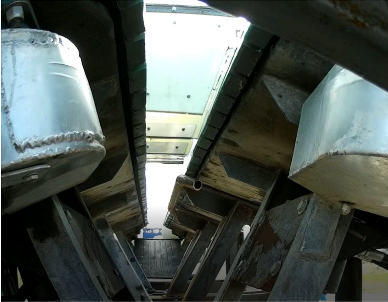
Figure 2. View from under the restrainer showing the negative contact bar for the left legs and the hot paddles suspended in the center of the restrainer.
