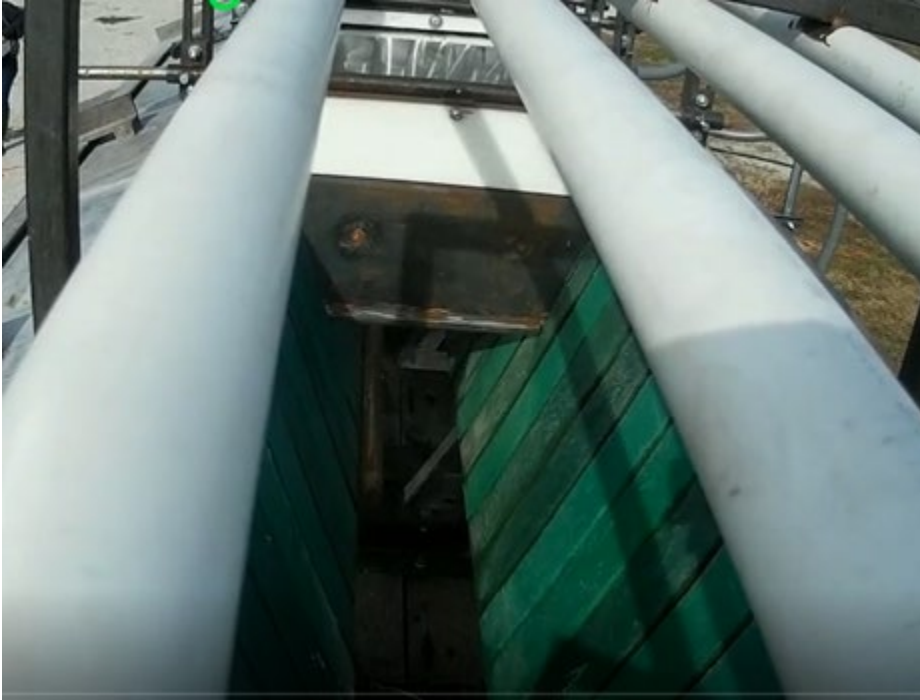
Figure 3. Top view of the negative contact bar with the original negative paddle still in place.
